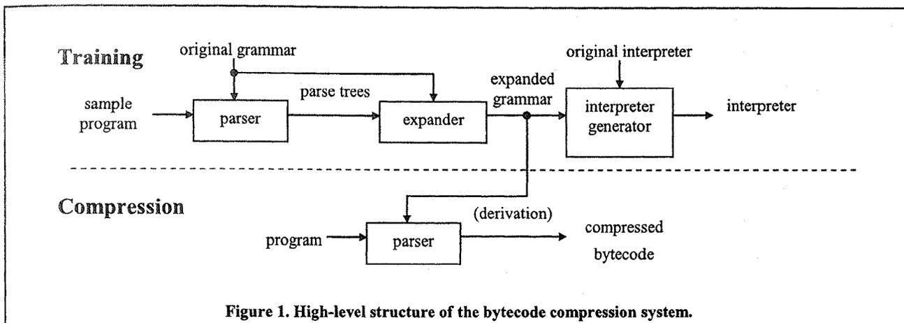
Figure 1. High-level structure of the bytecode compression system.
