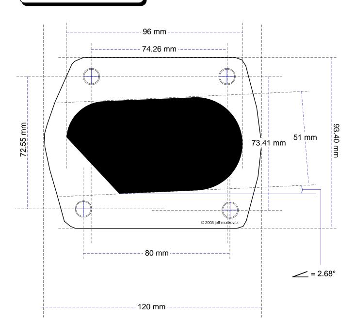
Note: The four mounting holes each have an inside diameter of 9 mm.
